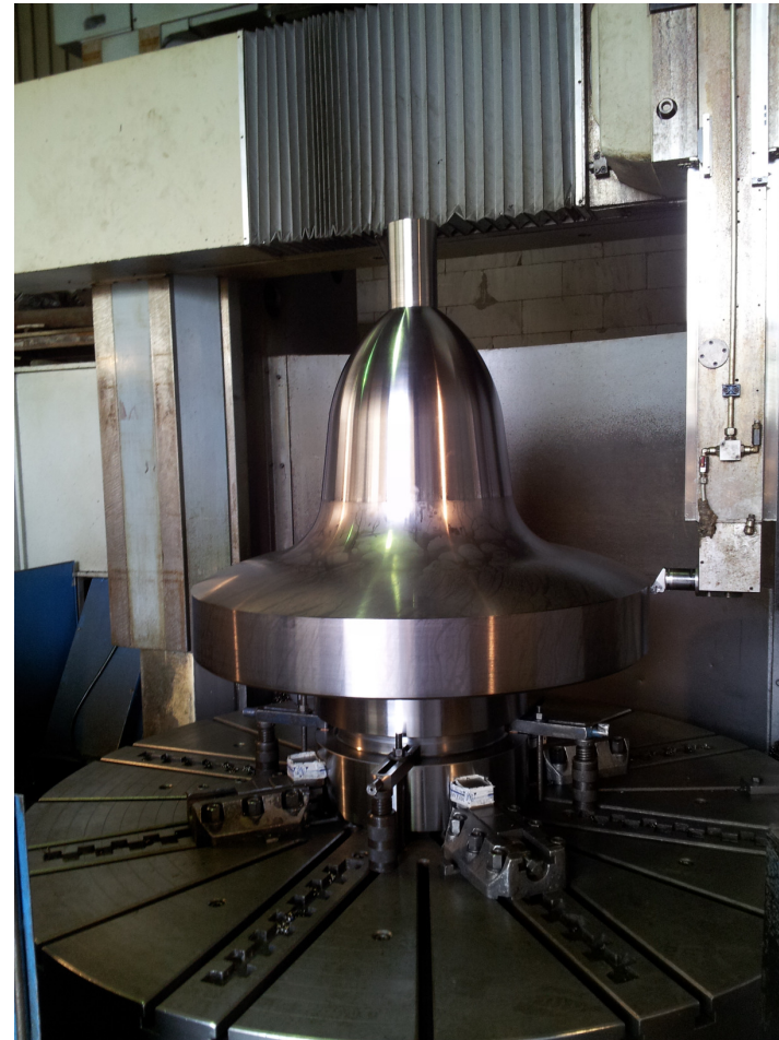
Punch for press Ø 1500 mm.
