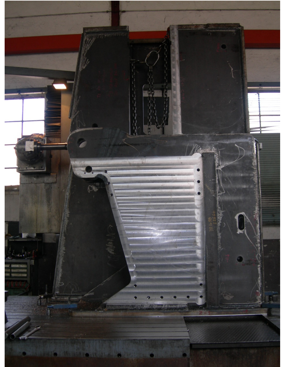
Shoulder for roll bending machine
