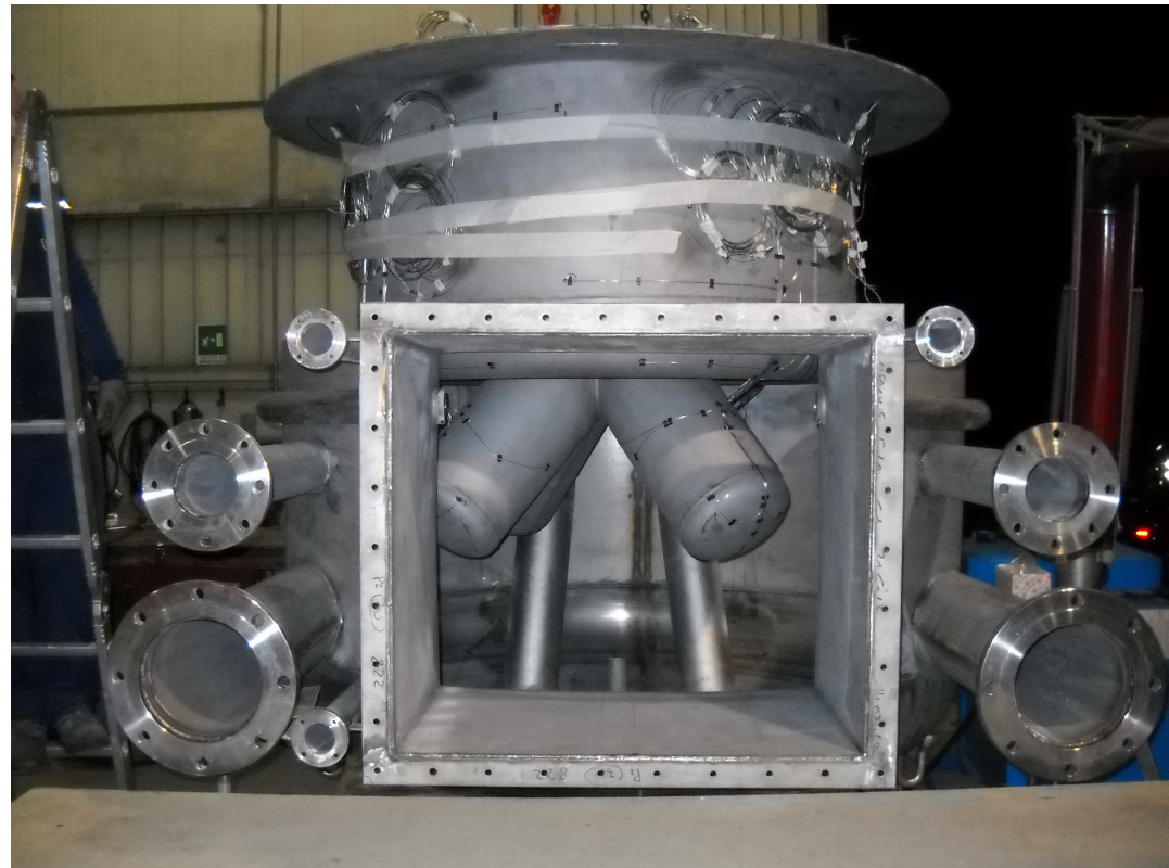
Receiver for solar tower plant
