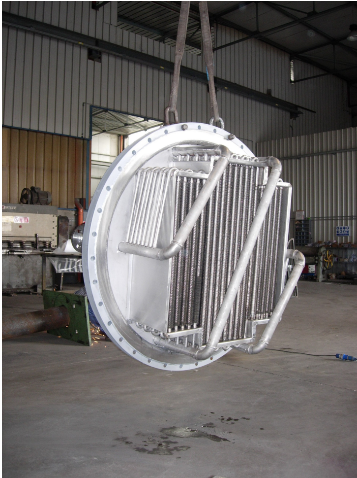
Gas dryer for polypropylene plant
