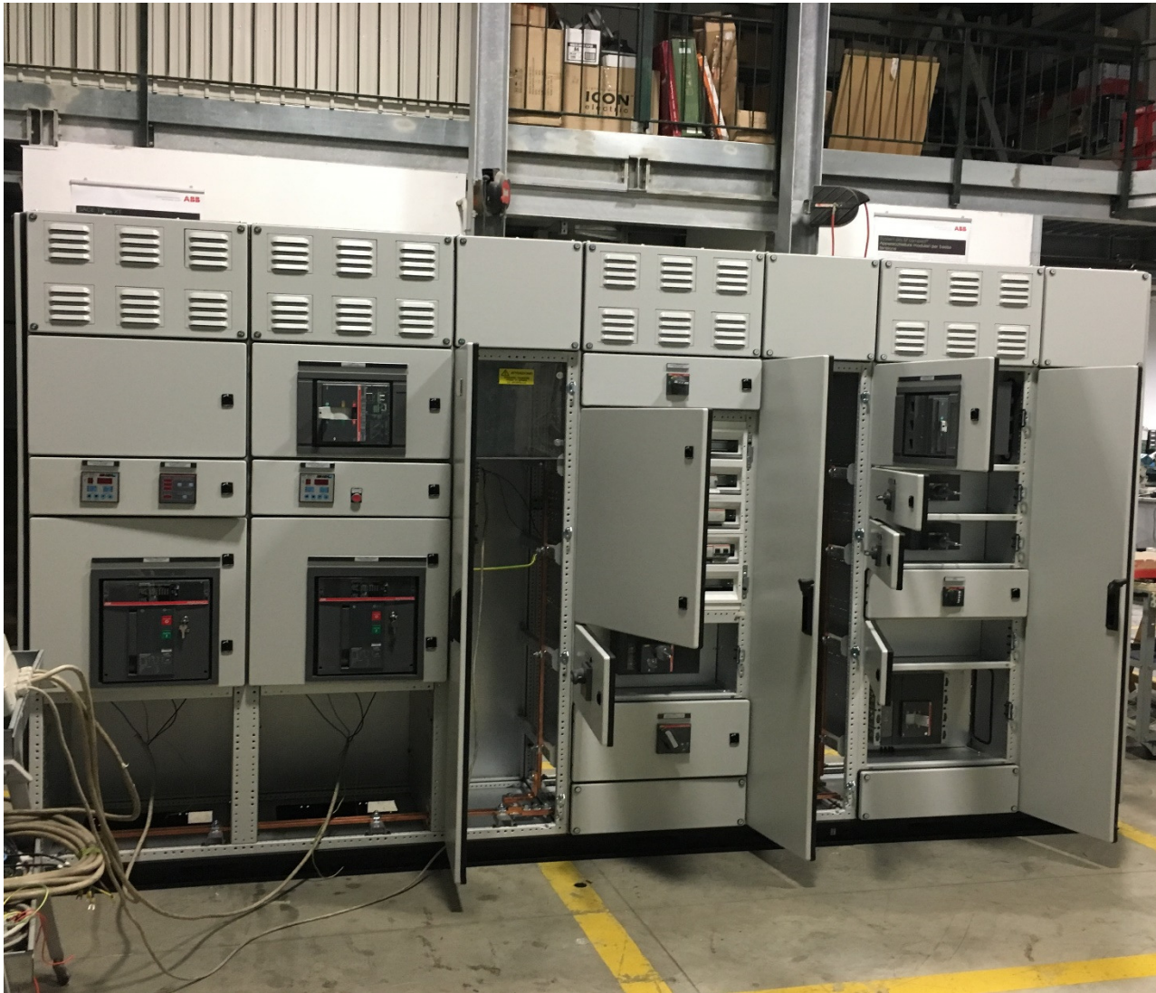
LV Distribution Panel for Power Center 2500A
