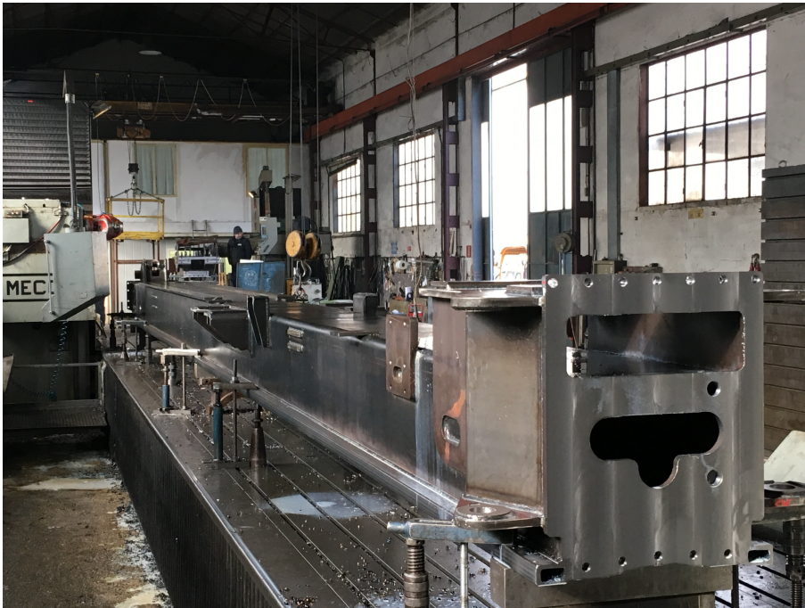
Frame for drilling machine (L= 13.000 mm.)
